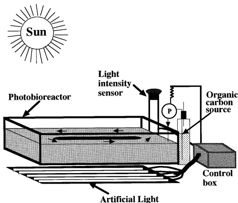
Fig. 4. A proposed low cost system for cyclic photoautotrophic-heterotrophic cultivation of photosynthetic cells, using solar and artificial light for continuous illumination during the photoautotrophic phase.
