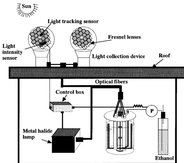
Fig. 1. An integrated system of solar light, artificial light and organic carbon supply for cyclic photoautotrophic-heterotrophic cultivation of photosynthetic cells.
