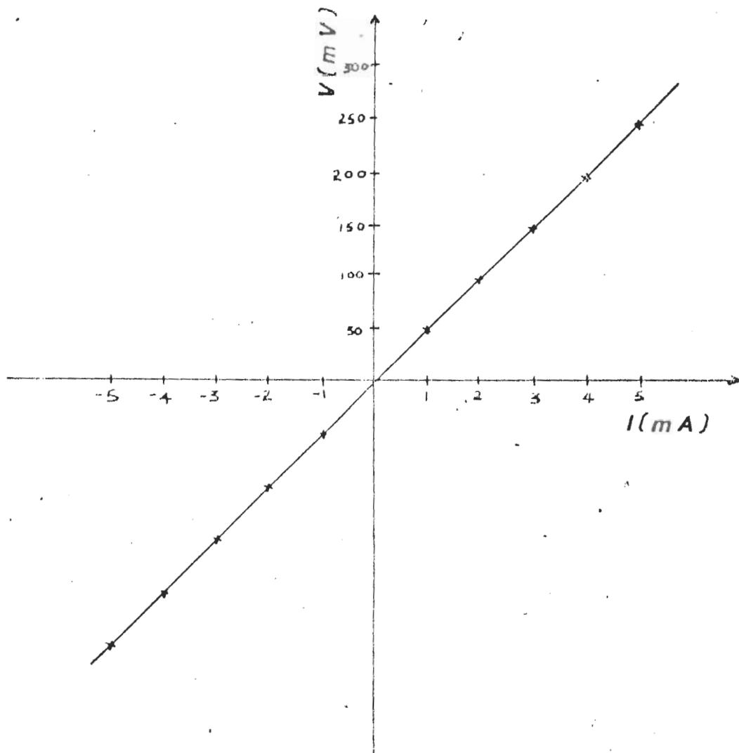
Figure 2: Linearity of the  $I$ - $V$  characteristics of electroplated silver layers on ITO
