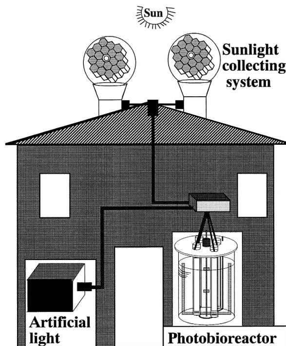
Fig. 7. Schematic diagram of the integrated solar and artificial light system for internal illumination of stirred tank photobioreactor.
