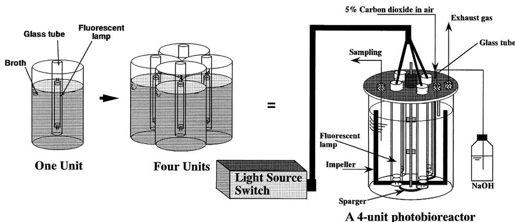
Fig. 6. Schematic diagram of an internally illuminated photobioreactor which can be used for efficient heterotrophic cultivation and photoactivation of photosynthetic cells.
